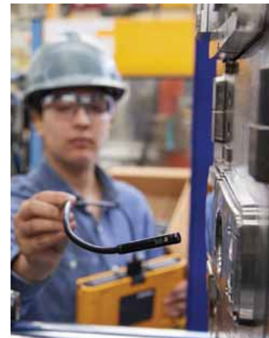
FLK-5.5MM/0.7M ART Articulating Camera FLK-9MM Scope Forward view, 20M probe reel
